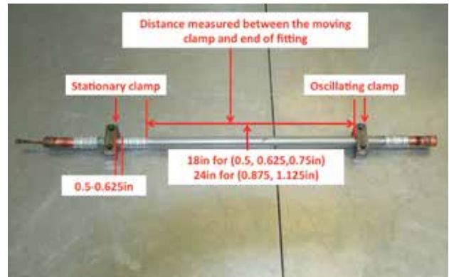
Test assembly of 0.5" and larger size tubes
